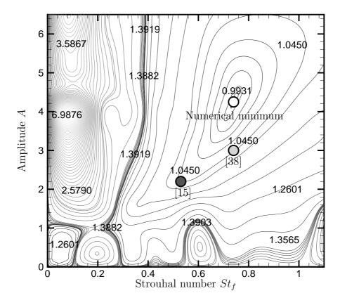
Fig. 2. Variation of the mean drag coefficient with A and  $St_f$  at Re = 200. Numerical minimum:  $(A_{\min}, St_{f_{\min}}) = (4.25, 0.74)$ ; [38]:  $(A, St_f) = (3., 0.75)$ ; [39] (not shown):  $(A, St_f) = (3.25, 1.13)$ ; [15]:  $(A, St_f) = (2.2, 0.53)$ .
