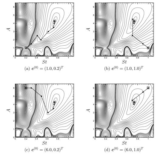
Fig. 11. Evolution of the control parameters during the optimization process for the different initial values  $c^{(0)}$ .
