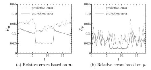
Fig. 5. Comparison of the prediction and projection relative errors based on  $\boldsymbol{u}$  and on p for the controlled cylinder wake flow  $(\gamma(t) = A\sin(2\pi St_f t))$  with A = 2 and  $St_f = 0.5$ ). The approximations  $\hat{\boldsymbol{u}}$  and  $\hat{\boldsymbol{p}}$  are evaluated for  $N_{\rm gal} = 14$ .
