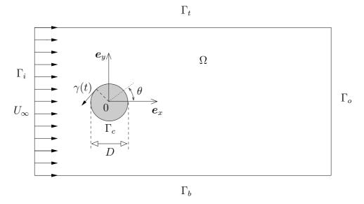
Fig. 1. Controlled flow configuration.
