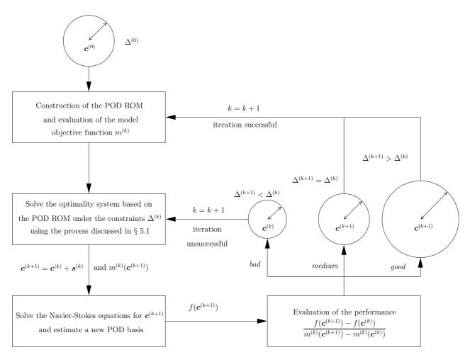
Fig. 3. Schematic representation of the TRPOD algorithm.
