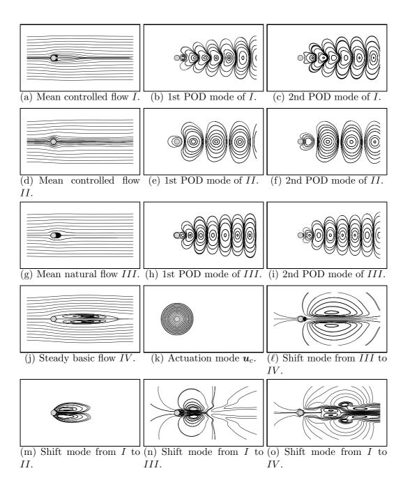
Fig. 6. Modes considered in the reduced-order control model (12) of the cylinder wake at Re=200. In all sub-figures, the flow is visualized with streamlines. Note that subfigure 6(d) looks like a potential solution and that subfigure 6(k) approximates a potential vortex.
