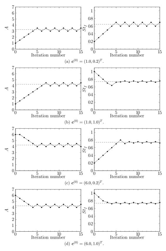
Fig. 9. Variations of the forcing amplitude (left) and Strouhal number (right) with respect to the iteration number. Results obtained with the adaptive method for  $\Delta_A = 0.5$  and  $\Delta_{St_f} = 0.1$ .
