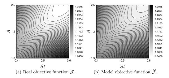
Fig. 8. Iso-values of the real and model objective functions associated to the mean drag coefficient. The same contour levels are used in the two figures.
