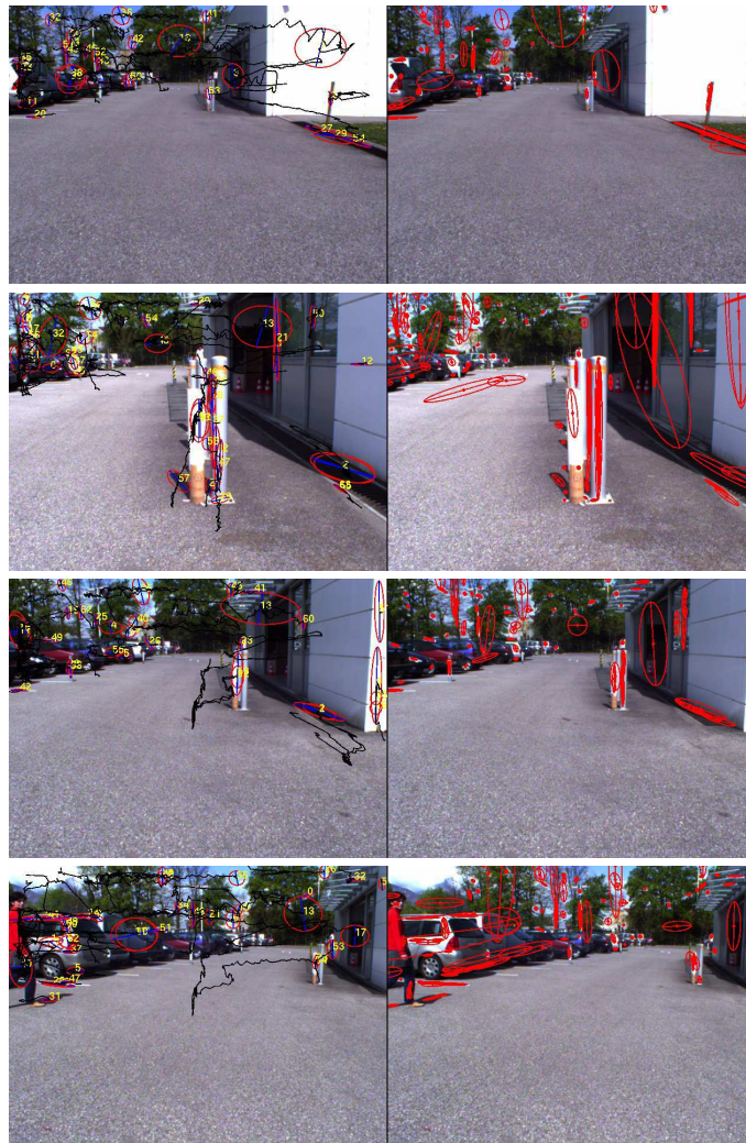
Fig. 5. Segment detection (right) and tracking (left) in an urban context. Red ellipses with blue axes represent the tracked segments, black curves represents segment's trajectories in the image.
