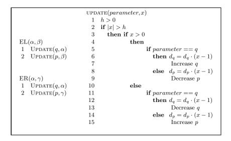
Fig. 17. Algorithms Fixed-Energy-And-Latency (EL) and Fixed-Energy-And-Reliability (ER). In EL, reliability is the free parameter and p and q are determined based on  $E_{feedback}$  and  $L_{feedback}$ . In ER, latency is the free parameter and p and q are determined based on  $E_{feedback}$  and  $R_{feedback}$ .
