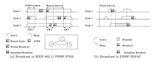
Fig. 2. Broadcast in PBBF with different sleep scheduling mechanisms.
