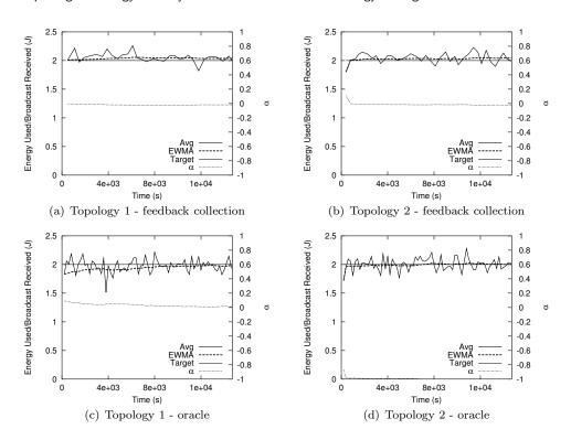
Fig. 20. Fixed-Energy-And-Latency (EL): Energy consumption under different topologies using feedback collection (a, b) and using an oracle (c, d).
