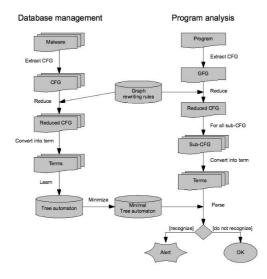
Figure 1: Design of the control flow detector
