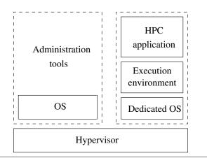
**Figure 1.** Running an HPC application in a dedicated domain under the control of a hypervisor.
