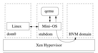
**Figure 4.** Stubdomain approach: qemu runs on top of Mini-OS in a specialized domain.
