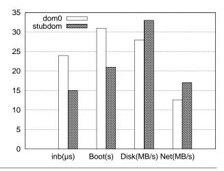
**Figure 5.** Performance of the fully virtualized guest, when qemu is running as a process in dom0, and when it is running in a *stub* domain: latency of guest I/O port access, guest boot time, throughput of disk and network.
