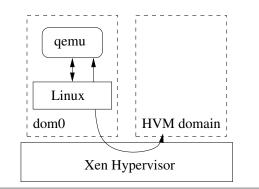
Figure 3. Traditional Xen approach: qemu, the device emulation component, runs as a process in dom0.
