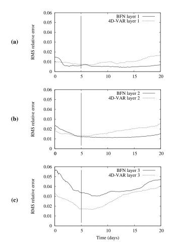
**Fig. 16.** Evolution in time of the RMS relative difference between the reference trajectory and the identified trajectories for the BFN (solid line) and 4D-VAR (dotted line) algorithms, versus time, for each layer: from surface (**a**) to bottom (**c**).
