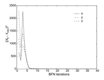
**Fig. 3.** Mean square difference between the observations and the BFN identified trajectory for the 3 variables versus the number of BFN iterations.
