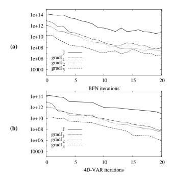
**Fig. 15.** Evolution of the 4D-VAR cost function and of the 3 gradients of the cost function in the 3 ocean layers for the BFN iterates versus the number of BFN iterations (**a**) and for the 4D-VAR iterates versus the number of 4D-VAR iterations (**b**) in the case of noisy observations.
