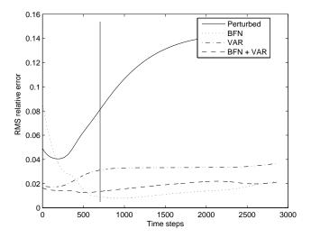
**Fig. 9.** Evolution in time of the RMS difference between the reference trajectory and the perturbed trajectory derived from the noisy observations of the system at time t=0 (full line), and between the reference trajectory and the identified trajectories for the BFN (dotted line), VAR (dash-dotted line) and BFN-preprocessed VAR (dashed line) algorithms, in the case of noisy observations (with a 5% RMS error).
