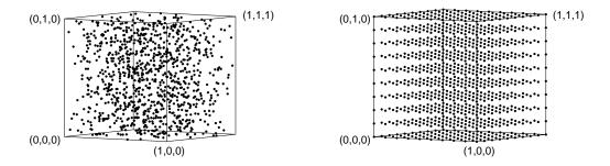
FIGURE 4. Test case 2. Input set  $(X_i)_{1 \le i \le N}$  is randomly generated, whereas the output set  $(Q_j)_{1 \le j \le N}$  is uniform, for 1000 particles. This configuration is similar to the one met in the SDM calculations.
