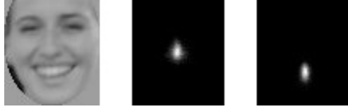
Fig. 3. Normalized face sample and likely locations for nose and mouth positions after normalization.
