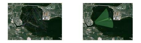
Fig. 5. Unsupervised Sensor Alignment: (Left) Color coded RADAR tracks at a port. (Right) The field-of-views of two high resolution cameras obtained using the proposed approach.
