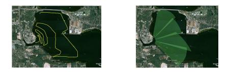
**Fig. 3.** Semi-supervised Sensor Alignment: (Left) A typical GPS track designed to be horizontal for better alignment. (Right) The field-of-views of four cameras obtained using the proposed approach at a port.
