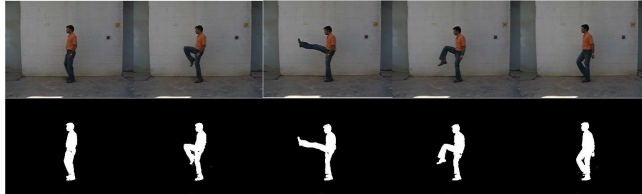
Fig. 5. An example action from our Outdoor Action Database with the corresponding background subtracted silhouettes.
