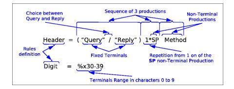
Fig. 2. Basic elements of a grammar
