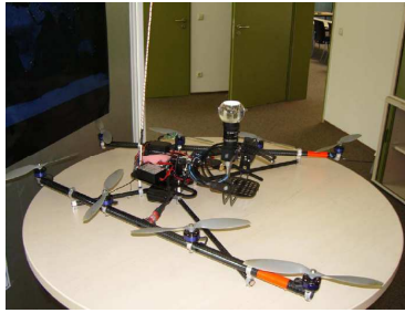
Fig. 6. Flying agent equipped with an omnidirectional sensor pointing upwards.
