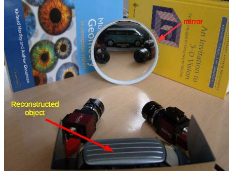
Fig. 4. Test setup to verify the approach with standard cameras for surgical applications.
