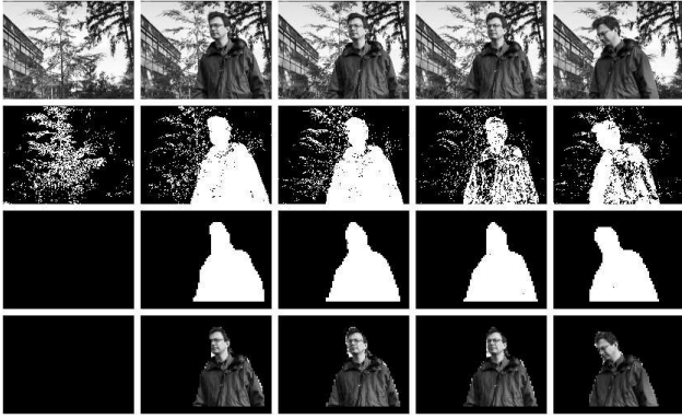
Figure 2. Experimental results on waving tree sequence. Morphological operators were not used in the results. The top row are the original images: 10 th , 246 th , 248 th , 252 th and 254 th frames. The second row are the results obtained by Mixture of Gaussians method (MOG). The third row are the results obtained by the proposed method, and the fourth row are the masked original images.
