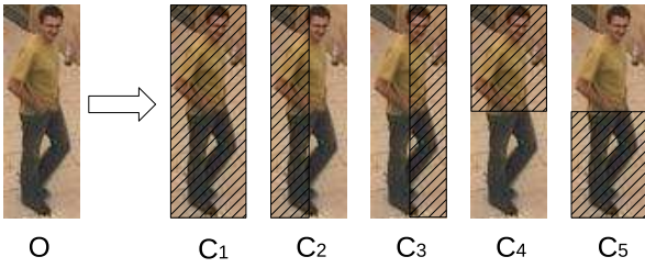
Figure 3. Object representation. Construction of the five covariance matrices from overlapping regions of an object feature image.
