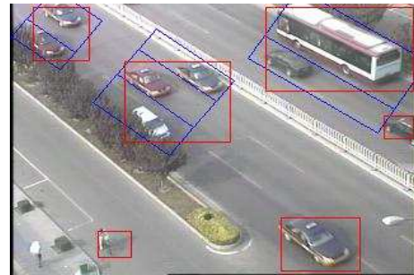
Figure 1. Some examples of single-vehicle blobs and multi-vehicle blobs. The red boxes are the results of GMM detector. The blue boxes segment the multi-vehicle blobs into single-vehicle blobs using our algorithm.
