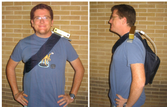
Fig. 5. Wearable stereo device used in our experiments that consists of a Bumblebee stereo camera and a small laptop, carried in a little backpack.
