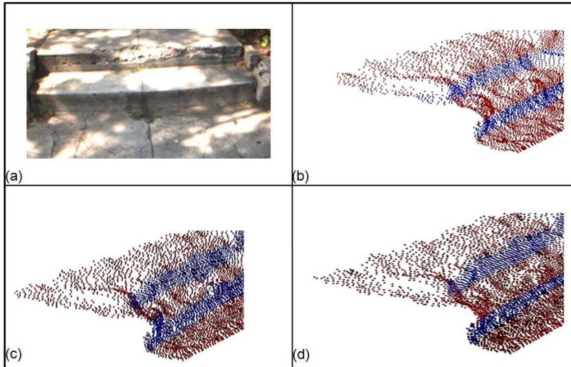
**Fig. 3.** Comparison of results obtained before tensor voting and after. (a) Original gray scale image (b) Input point-cloud manually clustered into horizontal (red) and vertical (blue) planes to generate ground truth (c) Segmentation after RANSAC processing only (d) Result after tensor voting
