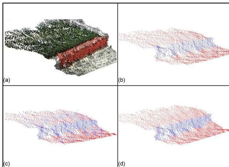
**Fig. 2.** Comparison of results obtained before Tensor Voting and after. (a) Original 3D point-cloud (b) Input point-cloud manually clustered into horizontal (red) and vertical (blue) planes to generate ground truth (c) Segmentation after RANSAC processing only (d) Result after tensor voting
