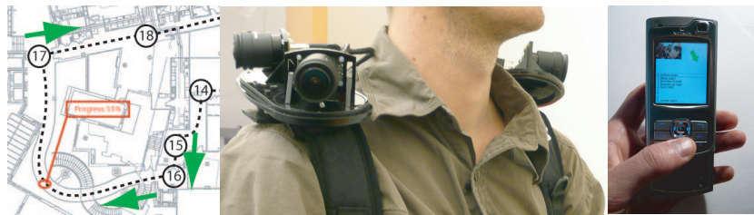
Fig. 2. Our operating scenario involves a human exploring a complex internal space (notional view at left; user path shown as dotted line). The user wears a multi-camera processing rig (center). At any point in time, the system provides audio information to the user about his/her global location in the place graph as well as user-centered directions toward the target destination.
