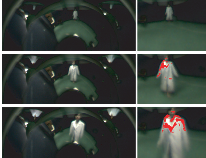
Fig. 6. Three examples of near object detection. The left column shows the inputs, while the right column illustrates the resulting perspective images where the area detected as near is marked in red.
