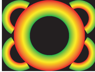
Fig. 5. Correspondence between the hyperboloidal mirror and surrounding paraboloidal mirrors when every ray is from infinity.
