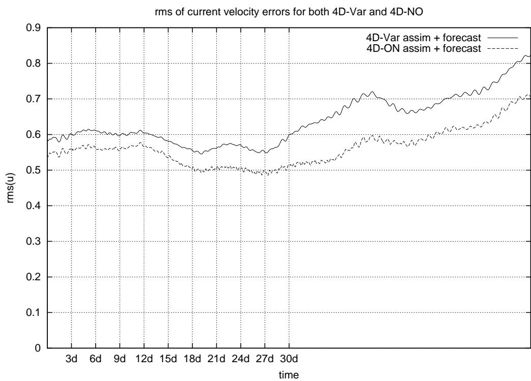
Figure 8: RMS of the error on current velocity for smoothed version of the 4D-ON compared to 4D-Var on assimilation window and one month forecast
