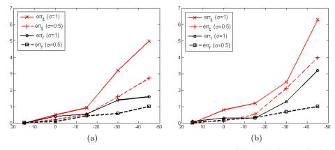
**Fig. 2.** Errors for  $\xi$  and f after non-linear optimization. (a)  $(\xi, f)=(0.96,360)$  (b)  $(\xi, f)=(0.80,270)$ . x-axis: vertical viewing angle of the highest 3D pattern point.
