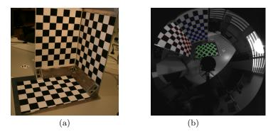
Fig. 3. (a) 3D pattern, (b) Omnidirectional image of the 3D pattern  $(1024 \times 768 \text{ pixels})$ .
