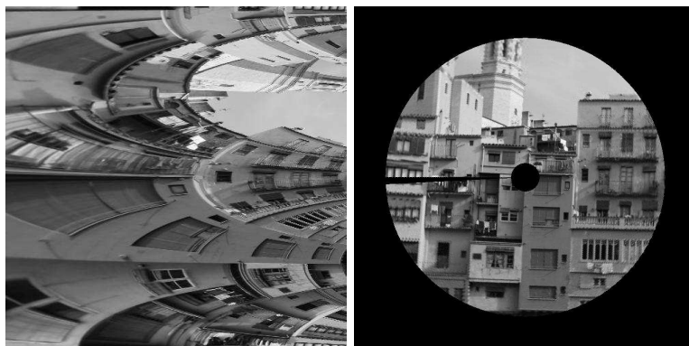
Fig. 1. Left: sample image acquired by a “log-polar” sensor. Right: calibrated image projected onto Z = 1
