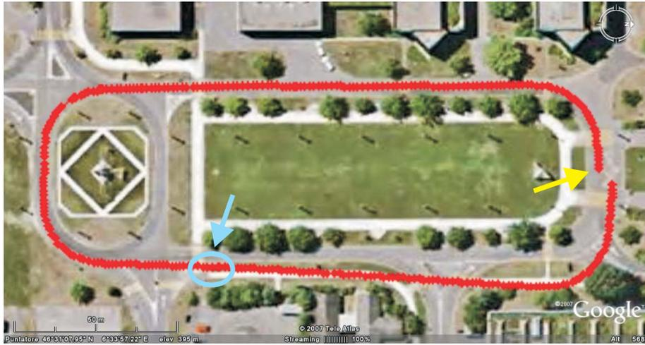
**Fig. 6.** The estimated path (before loop closing) superimposed onto a Google Earth image of the test environment. The scale is shown at the lower left corner.
