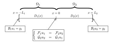
Figure 1: Decomposition of the spatial domain  $\Omega$  into two non-overlapping subdomains.
