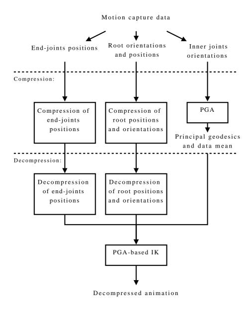
Figure 1: Flow diagram for the compression pipeline
