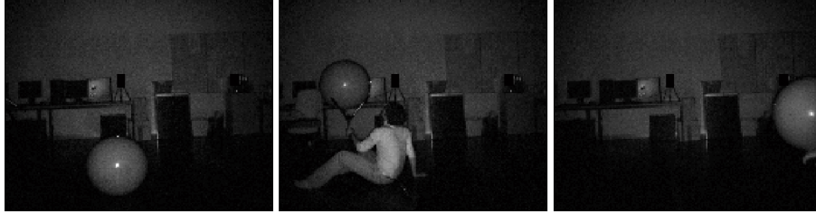
Fig. 5. ToF camera Swiss Ranger 3100 intensity image sphere center highlights. To detect the highlight robustly and automatically, we apply a simple Region of Interest (ROI) tracking method.
