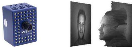
Fig. 1. Left: A ToF camera, Swiss Range 3000. Right: Typical output from the sensor: an intensity (amplitude) image and a 2.5D depth image. (Courtesy of MESA imaging.)
