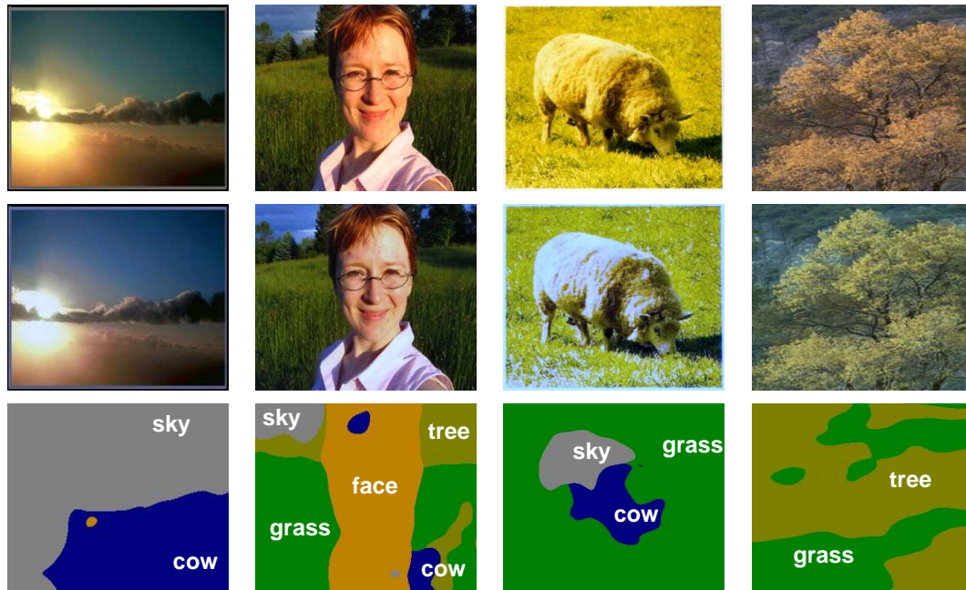
Figure 4. Example of pixel classification. First row: input images. Second row: illuminant corrected images selected by our approach. All four are based on a top-down illuminant hypothesis. The hypotheses are based from left to right on the classes sky, face, grass, and tree. Third row: pixel classification results based on the images in the second row.
