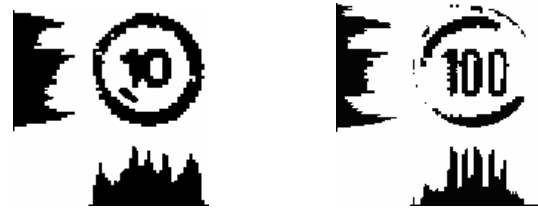
Fig. 3. Histograms of binarized speed limit signs
