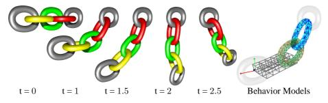
Figure 5. Animation of a chain combining a FEM model, a mass-spring model, a FFD grid, and a rigid body.
