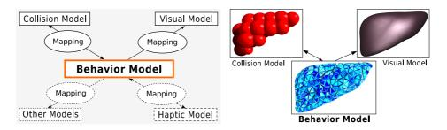
**Figure 1.** Illustration of the multi-model representation in SOFA. *Left*: possible representations for a simulated object, with the Behavior Model controlling the update of the other representations through a series of mappings. *Right*: examples of these representations for a liver model. Notice how the Visual Model is more detailed than the Behavior Model and how the Collision Model relies on a very different representation.
