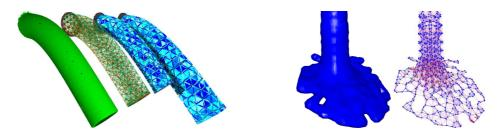
Figure 4. Left: surface of an actual soft cylindrical object compared to a mass-spring, co-rotational FEM, and linear FEM models, under the same constraints. Right: a fluid modeled in SOFA using a SPH method.
