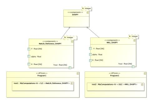
Figure 4: Instanciation of the parameterized component
