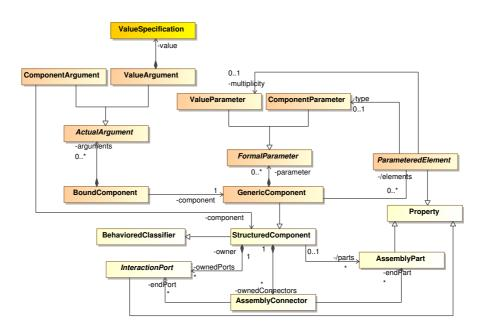
Figure 7: The Generic Component Modeling package of the MARTE metamodel after introduction of genericity
