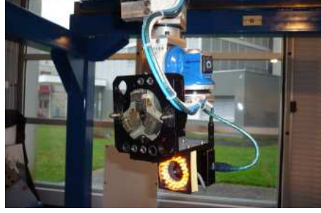
Figure 14: Camera and light-ring mounted on the robot end-effector.
