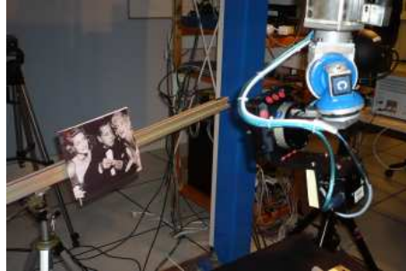
Figure 16: View of the lighting, the camera and the object to track. The object (a photo) is attached to a motorized rail that allows to control its motion.
