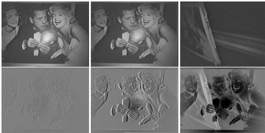
Figure 17: First experiment: Tracking considering the interaction matrix under temporal luminance constancy hypothesis. As can be seen the tracking task failed quickly. First row shows the image acquired by the camera while \mathbf{I} - \mathbf{I}^* is shown on the second row.
