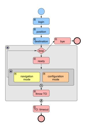
Fig. 3. Functionality workflow of the GPS Web service
