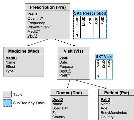
Figure 3. Database schema and SubTree Key Tables.
