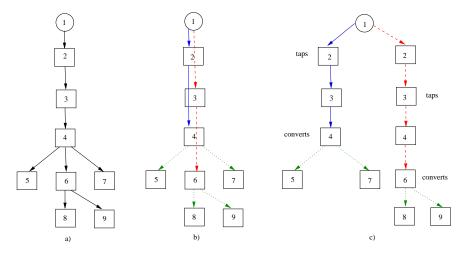
Figure 14: Example of optimal virtual toplogy with at most two wavelengths per fibers and one tap operation.
