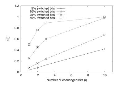
Figure 23: p(x,i) when 5, 10, 25 and 50% of the 1-bits are switched. p(x,i) increases as the lying percentage and the number of challenged bits increase.
