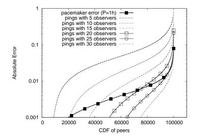
Figure 19: A comparison between Pacemaker and the ping-based system for exponential distribution. Pacemaker performs better than a ping-based system with 20 observers for each peer.
