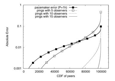
Figure 18: A comparison between Pacemaker and ping-based system for uniform distribution. Pacemaker is equivalent to a ping-based system that uses 5 and 10 observers for each peer.
