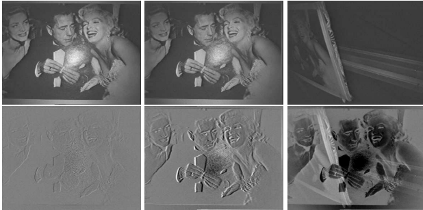
Figure 6. First experiment: Tracking considering the interaction matrix under Lambertian hypothesis. As can be seen tracking failed quickly leading to incoherent robot motion. First row shows the image acquired by the camera while \mathbf{I} - \mathbf{I}^* is shown on the second row.
