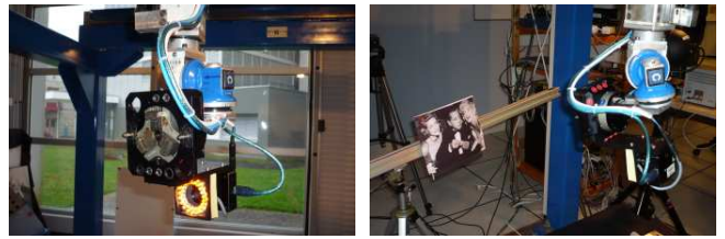
Figure 4. Camera and light-ring mounted on the robot end-effector and view of the object to track and of the camera. The object (a photo) is attached to a motorized rail that allows to control its motion.
