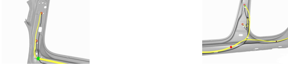
Figure 3: Virtual prototyping: positioning of the two opposite extremities of a cable bundle. Its different parts are assembled with fusion constraints.
