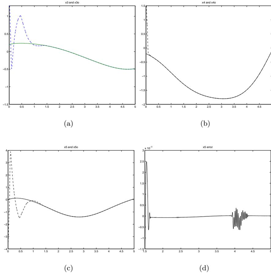
**Fig. 1.1.** State (solid line) and estimation (dotted line)
