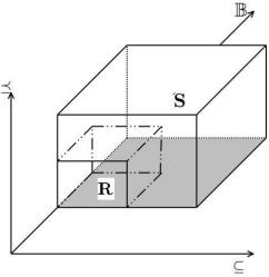
Left, the relation between two process-filters  $\mathbf{R}$  and  $\mathbf{S}$  which represent the same set of constraints but on a different set of controlled variables:  $\mathbf{R}$  is less wide than  $\mathbf{S}$  because the set of processes represented by R under the given constraints is included in that of S.
