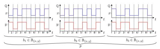
**Definition 2.** [Process] For **X**, a finite set of variables  $(\mathbf{X} \subset_{\ell} \mathcal{V})$ , an **X**-process p is a nonempty set of **X**-behaviors. The *empty process* (a  $\emptyset$ -process) is a unique process designated by  $\Omega =_{\Delta} \{\emptyset\}$  and must be distinguished from the *blocking process*  $\mho =_{\Delta} \emptyset$ .
