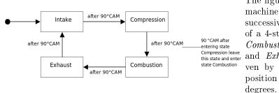
The figure represents a state machine that denotes the successive operation modes of a 4-stroke engine : *Intake*, *Combustion*, *Compression*, and *Exhaust*. They are driven by the camshaft whose position is measured in angle degrees.
