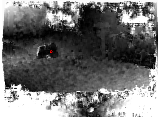
Fig. 10. Estimation of the parallax-based rigidity constraint with respect to the point circled in red. In black, the points consistent with the reference one according to the constraint given by (8).
