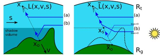
**Figure 1: Our method.** Left: the reference solution includes single-scattering (a) and multiple-scattering (b) integrated from  $\mathbf{x}$  to  $\mathbf{x}_o$ , all accounting for occlusion. Right: our approximation. Integration is done from  $\mathbf{x}$  to  $\mathbf{x}_s$ , ignoring occlusion (implicit via the use of  $\mathbf{x}_s$ ). (a) is unchanged. (b) is affected by ignoring occlusion of secondary scatters (this yields both positive and negative bias, and effect is small anyway).
