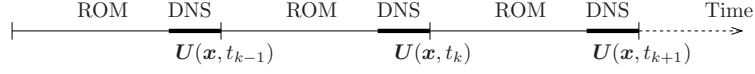
Figure 24: Schematic representation of the hybrid method DNS-POD ROM to improve the POD subspace.
