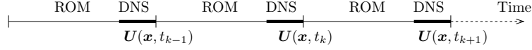
Figure 24: Schematic representation of the hybrid method DNS-POD ROM to improve the POD subspace.
