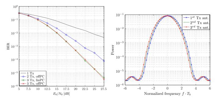
Figure 6: Left: Simulated bit error rate (BER) over a Rayleigh fading channel; Right: Power spectral density of the linPC analyzed with the Welch algorithm.
