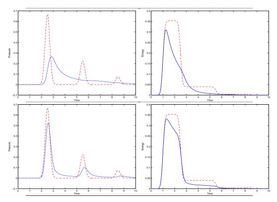
Figure 3.2: Influence of the parameter  $\eta$  in a cylinder. Top:  $\eta = 0.5$  in blue plain line, compared to the reference  $\eta = 0$  in red dotted line. Bottom:  $\eta = 0.11$  in blue plain line, compared to the reference  $\eta = 0$  in red dotted line. The pressure signals at the output versus time are shown on the left, whereas the wave energy in the cylinder is plotted versus time on the right.
