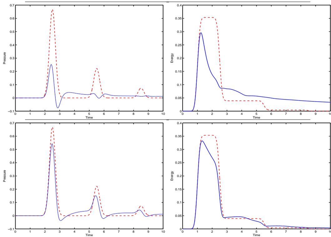
Figure 3.1: Influence of the parameter  $\varepsilon$  in a cylinder. Top:  $\varepsilon = 1$  in blue plain line, compared to the reference  $\varepsilon = 0$  in red dotted line. Bottom:  $\varepsilon = 0.2$  in blue plain line, compared to the reference  $\varepsilon = 0$  in red dotted line. The pressure signals at the output versus time are shown on the left, whereas the wave energy in the cylinder is plotted versus time on the right.
