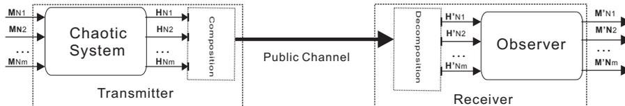
Fig. 1. Scheme for multiple secure communication system
