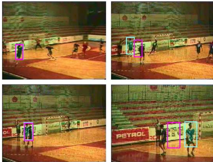
Figure 5: Probabilistic tracking of size changes during occlusion in clutter. Handball sequence extracted from the HandballC.avi file of the CVBASE'06 dataset, images #10828, 10883, 10948 and 10986. A particle filter is used with camera motion compensation and with (in blue) or without (in magenta) adaptation. When the adaptation is on, it is performed as soon as no partial or total occlusion is detected.
